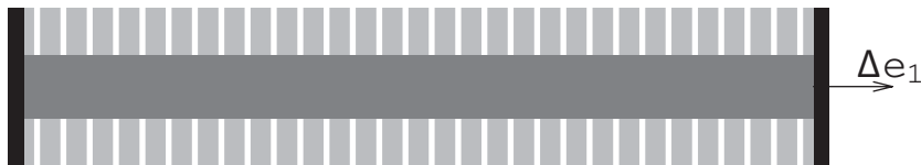
Figure 6.8. Transverse periodic cracking
